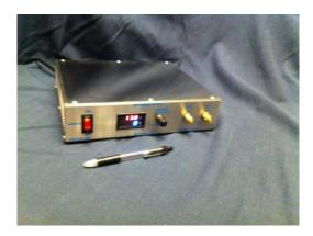
Output Voltage is adjustable from 8.75 to 14.5 Vdc.
